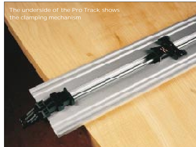
The clamping mechanism has three positions: up to release, in the middle to tighten, and down for extra tight
