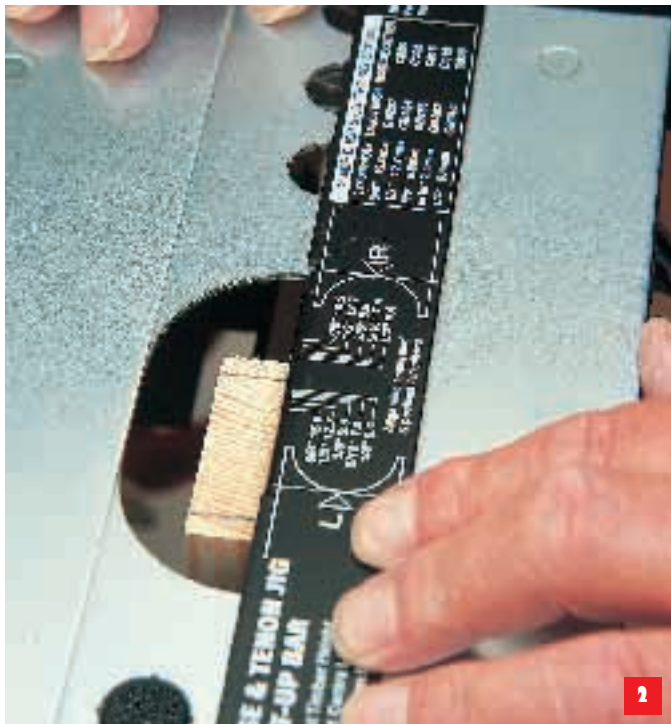
The jig being set up for a tenon
