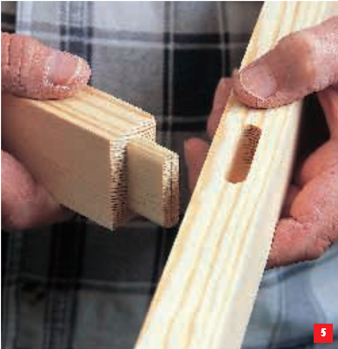
The two halves of the joint, showing the rounded ends of both mortise and tenon
