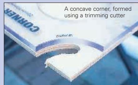
A concave corner, formed using a trimming cutter
