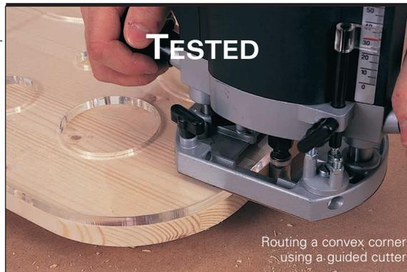
Routing a convex corner using a guided cutter
