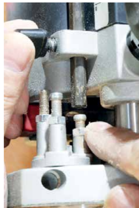
The rotating turret and depth post are simple but very effective for many routing jobs
