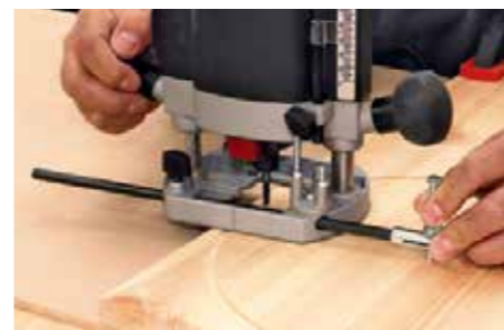
Also supplied in the kit is the trammel point for circle and arc work
