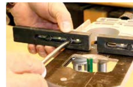
The sliding fence facings allow full support for different sized bits and applications
