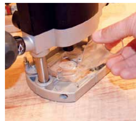
A clip-in dust kit is supplied to control the dust and help keep the work area clear as you rout
