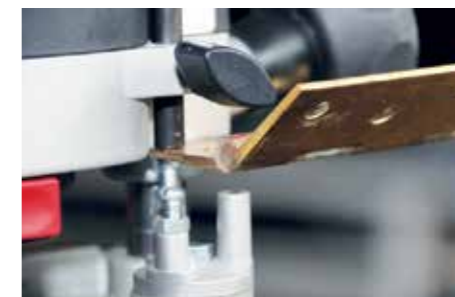
You can use the turret to gauge against fittings such as hinges...
