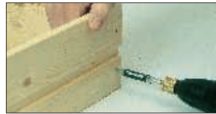
The magnetic screw holder makes a big difference to the time it takes to complete a job
