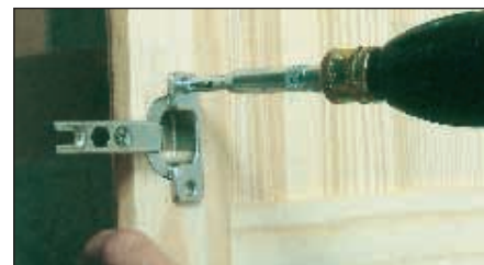
The drill bit guides will centre the drill in a hinge hole
