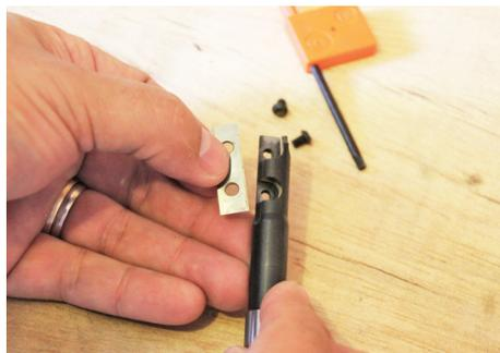
▲ The cutter slides into the body, self setting for fast swapping
