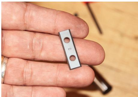
▲ These replaceable bits have dual cutting edges as well as a bottom plunge cut
