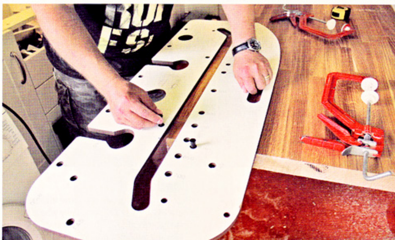
▲ The jig is positioned by pushing in the pins in the correct holes to suit the cut
