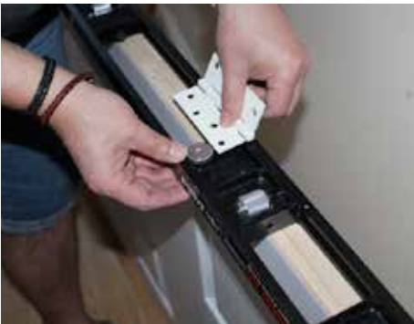
▲ These discs have three positions for conventional leaf widths or can be set to suit
