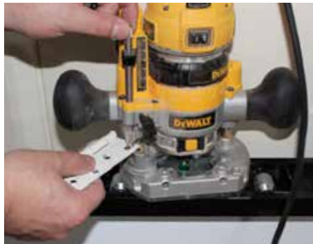
▲ Use the leaf as a gauge to set the router to remove the correct thickness
