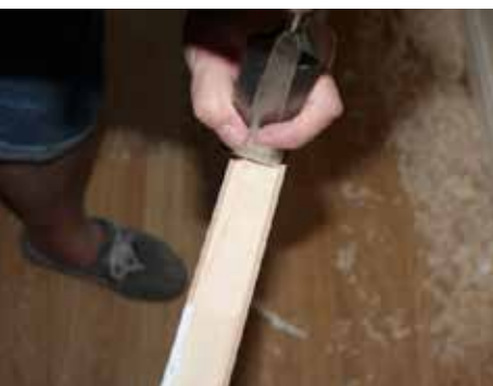
▲ The jig leaves rounded corners, easily removed with a sharp chisel
