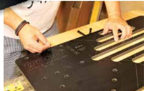
▲ Alternatively set the pins on the 90° setting for a diagonal pattern
