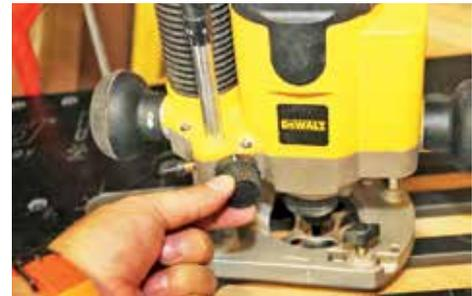
▲ Set the depth by plunging the cutter to the worktop and zeroing the post
