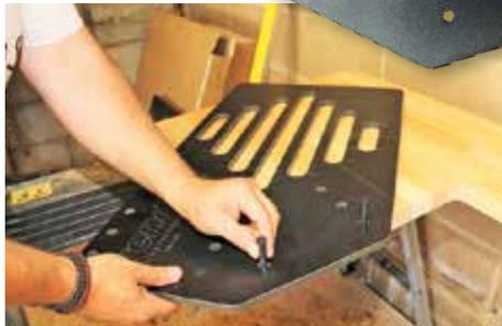
▲ Use the pins on the 45° position for a parallel design
