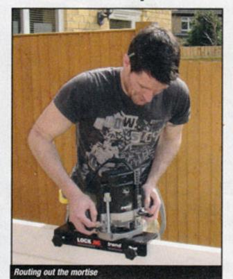
to be fitted with the 30mm guide bush and it is supplied with and a 12mm cutter with an overall length of 115mm. It should be noted that I used different routers for the lock and hinge jigs. With the use of a guide bush collar supplied with the lock jig it is possible to use one router for both operations without changing the guide bush.
