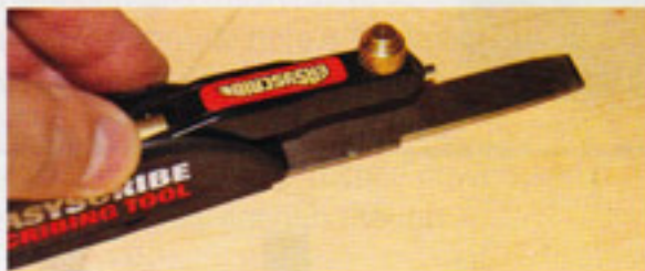
The leg extends to suit the work being scribed
