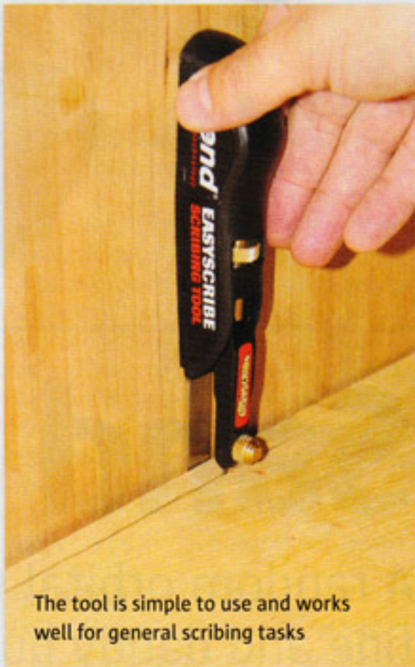
The leg extends to suit the work being scribed
