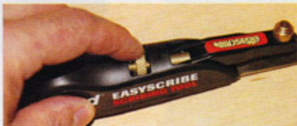
The legs are adjusted via this wheel
