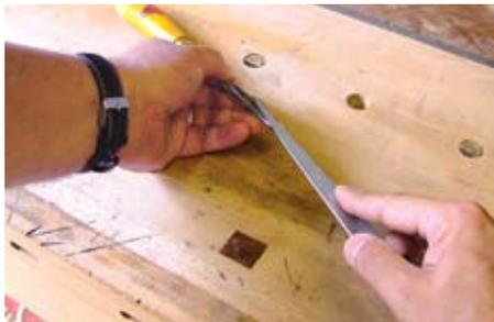
▲ The curved face is ideal for gouges or curved edges
