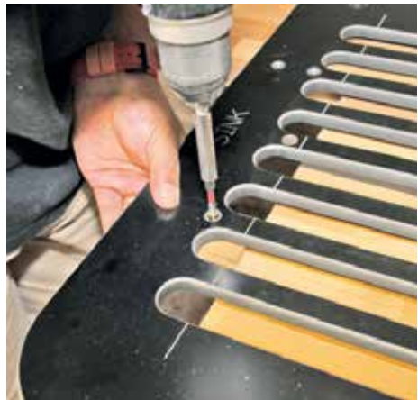
▲ You can fit a couple of stops for quicker setup
