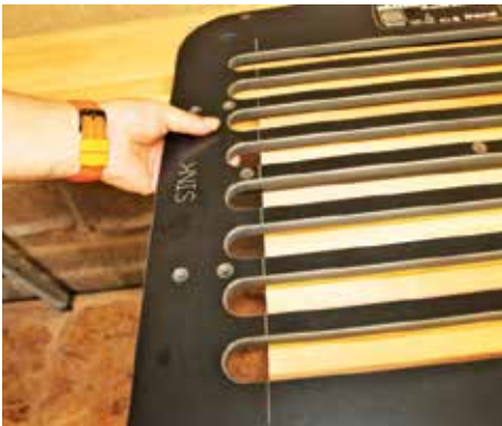
▲ The jig has three tapered packers fitted to get the correct fall and a datum line sets it correctly for a full-length slot
