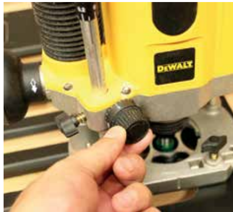
▲ ...then back off the plunge post to the correct cutting depth
