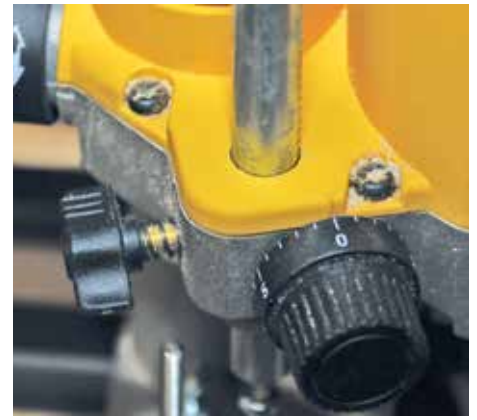
▲ Set the depth by plunging the cutter and zeroing...
