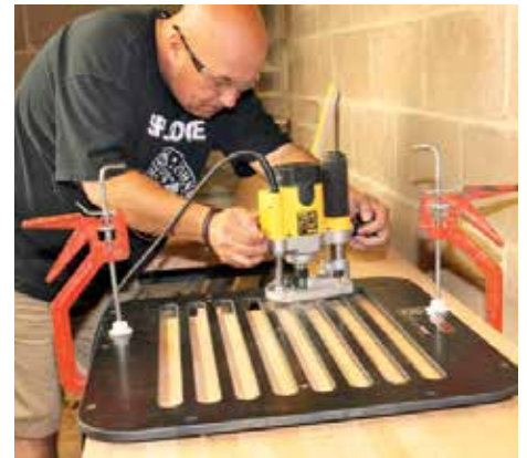
▲ Starting at the innermost slot helps eliminate mistakes
