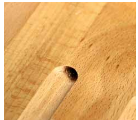
▲ Ideally a few test cuts will help eliminate the scorching shown here
