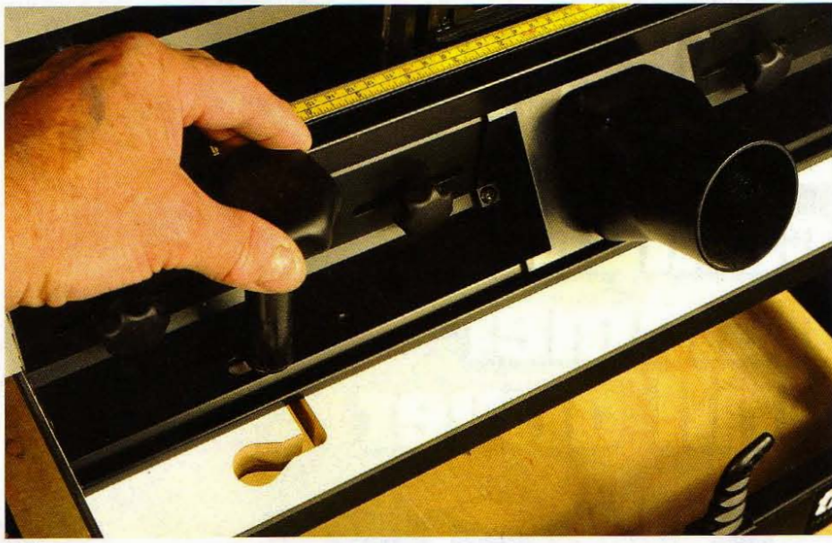
Once the lock knobs are undone, slide the fence backwards and off to the side, then you can lift the fence clear of the table for table routing with the lead-in pin only
