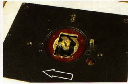
All the holes for Trend router mounting, the Quick Raiser and lead-in pin are precision machined into the insert plate
