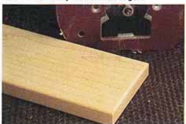
34 Machine up the drawer fronts with a tiny radius on all edges.
