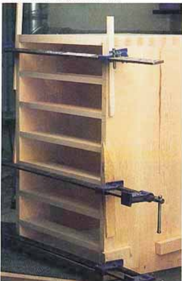
26 Hold it together with sash cramps checking for squareness.
