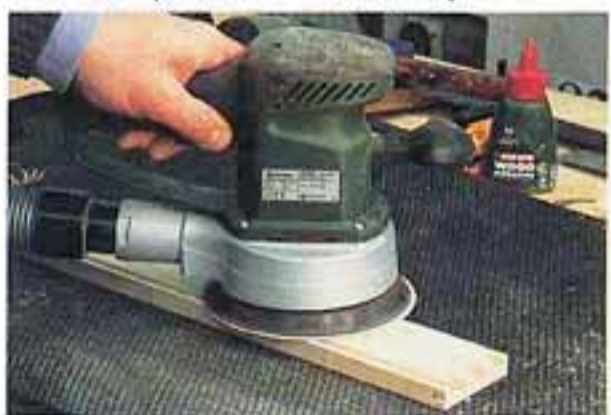
31 Sand the inside of the drawer components before assembly.
