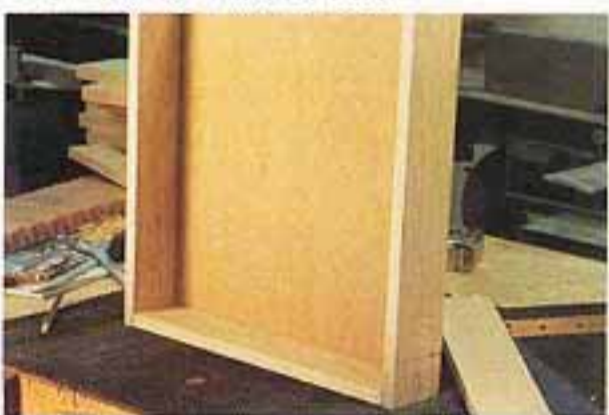
32 Assemble each draw with its 6mm MDF base.
