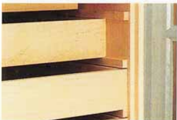
39 Check that the drawers finish a few millimetres clear of the back.
