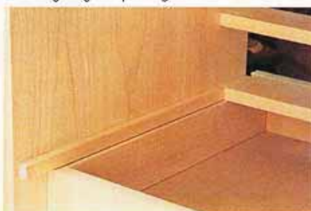
37 Fit the drawer runners by gluing and pinning them to the sides.
