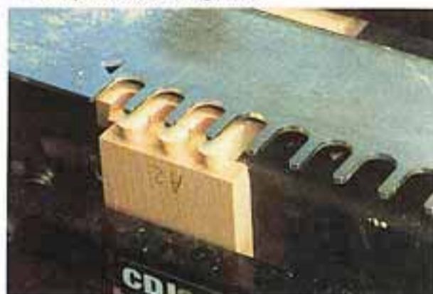
28 Both parts of the lap dovetail joint are cut together.
