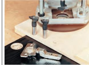
Our new range of machine bits are for use in portable plunge routers. These specially designed machine bits have a new form of scriber to allow use at high speeds, Max. 20,000 RPM. For accurate repetitive routing, a template and guide bush fitted to the router base should be used. Ref. 105 group.
