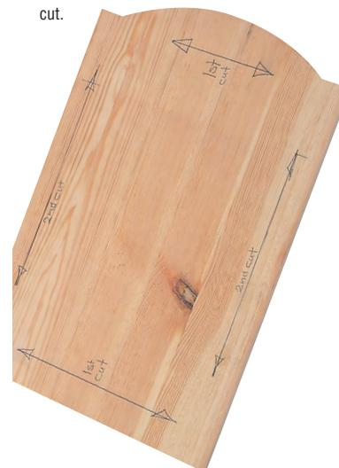
If the cutter persists in tearing the grain, score across the cut line with a sharp knife, the width of the cutter in from the edge of the workpiece (i.e. distance from the outer tip of the cutter to the bearing or fence).
