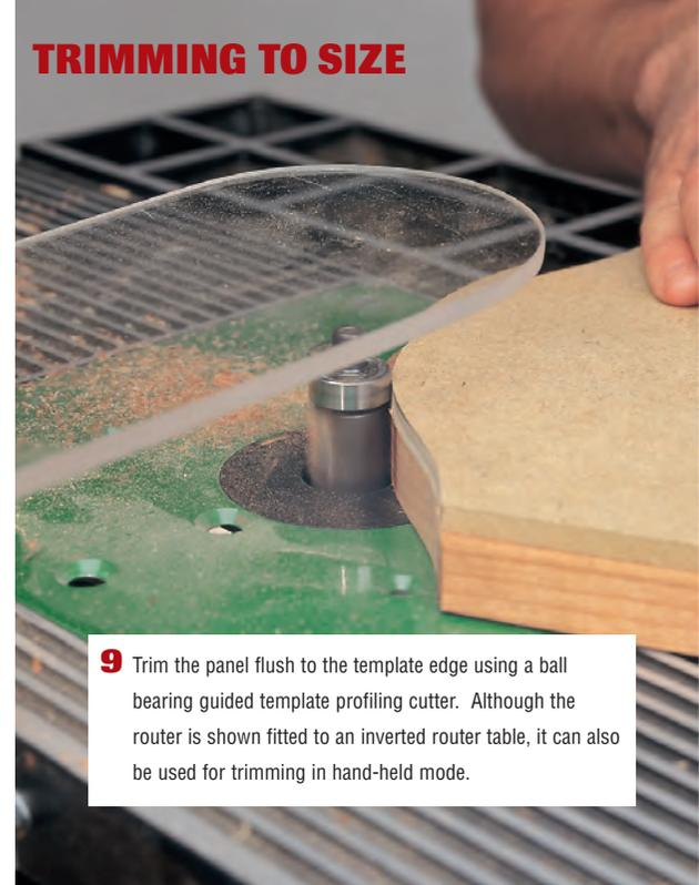
9 Trim the panel flush to the template edge using a ball bearing guided template profiling cutter. Although the router is shown fitted to an inverted router table, it can also be used for trimming in hand-held mode.
