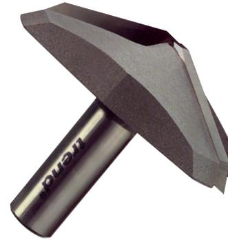
Large diameter horizontal raised panel cutters are used for moulding straight edges against the table fence. It is advisable to use them only in table mounted variable speed routers at their recommended safe speed. Cutters above 50mm in diameter, should be used at speeds not exceeding 18,000 rpm, above 70mm diameter at 16,000 rpm and above 80mm in diameter at 12,000 rpm.
