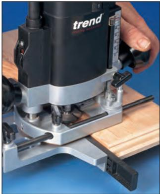
Edge moulding using a side fence.
