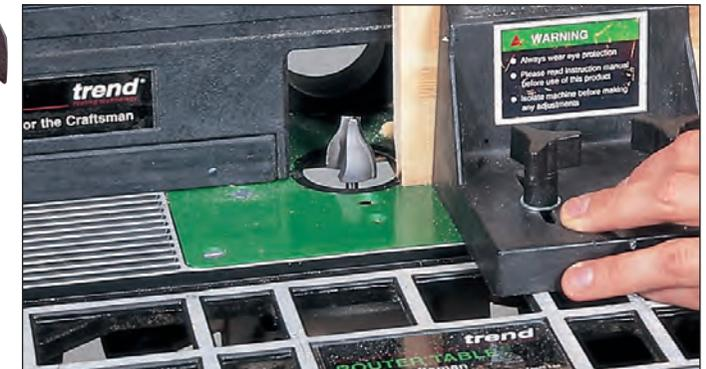
Positioning the vertical front support block
