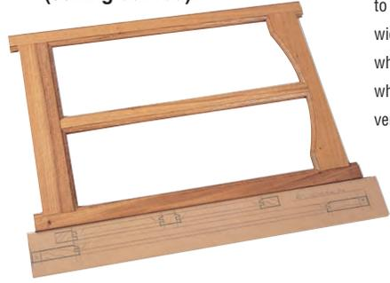
1 For solid timber frames and panels, add to the length of the panel
