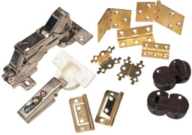
The size and type of hinge chosen will depend on the size and weight of the door itself. With flap hinges the thickness of the door stile in relation to the flap width will dictate the hinge size used. Economy lay-on hinges are only suitable for lightweight doors up to 450mm wide. Concealed hinges will support larger and heavier doors and are fully adjustable once fitted.
