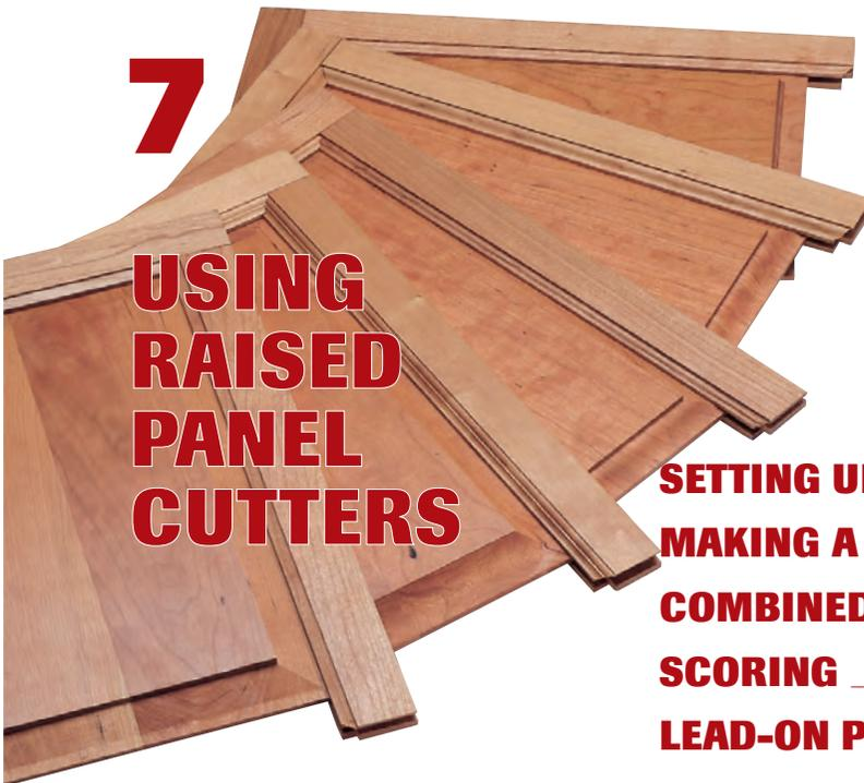
**R**aised panel cutters are used to cut away the panel edge to fit into the rail or stile groove, producing a decorative bevel, radius, ogee or ovolo moulding.
