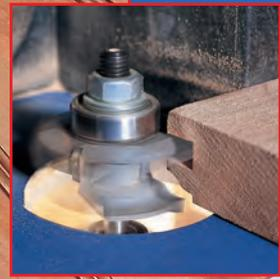
*A guide to using profile scribing and raised panel cutters*
