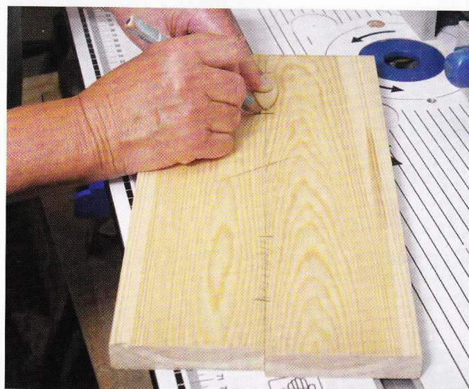
3 Boards being marked for biscuiting
