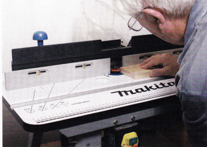
6 The cutter being set to the middle of the board
