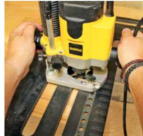
▲ With the jig set and clamped for the drip, the first cut is made
