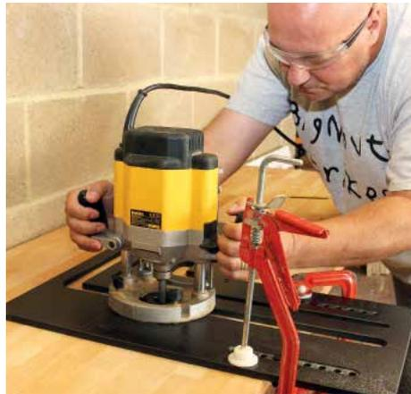
▲ The cut is made in two halves, working from the left inwards to avoid breakout
