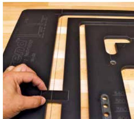
▲ The jig comes with a datum gauge block to correctly set it up to the layout lines
