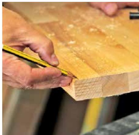
▲ The drip groove is formed by first marking the backset start and finish point for the cut
