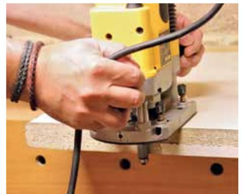
▲ A second pass then removes the rest of the lipping for a clean smooth surface
