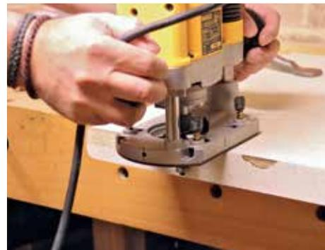
▲ Set the router to make the first pass just over half the depth of the worktop
