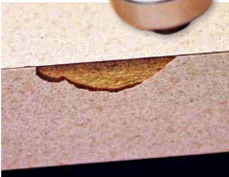
▲ A damaged lipping can be a pain to remove and replace
