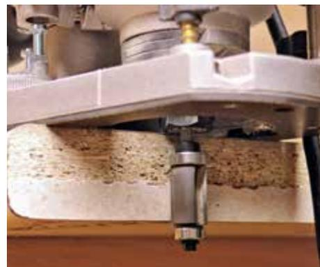
▲ Set the router so the top bearing engages the new rebate and is deep enough to remove the rest
