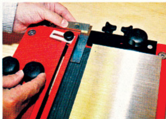
▲ The backstop is set for square or with a bevel to accommodate out-of-plumb work
