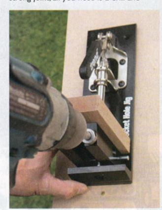
some self-tapping screws. The screw acts as an internal clamp holding the joint together, so you don't need any glue either, although I would recommend this as a belt and braces approach.
