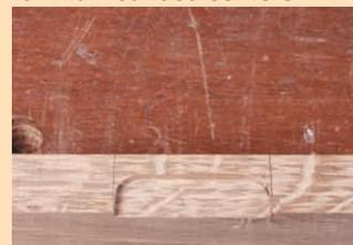
against the edge, where it automatically aligns itself. One sharp blow with a hammer squares the corner and the waste is lifted out with a chisel.
