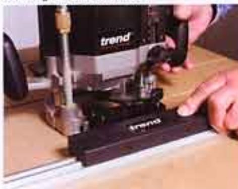
The router base showing the bottom end of the Quick Raiser (upper left)
