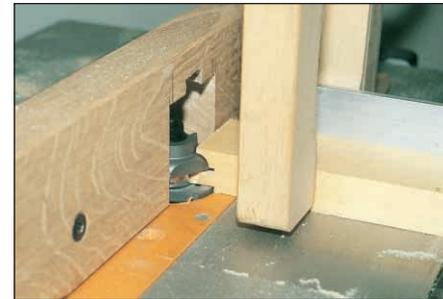
Grooving a shaped edge using the variable kerf groover
