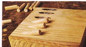
Glue the plugs into their pre-drilled holes
