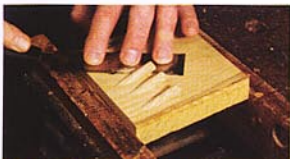
Cut off the excess when the glue has dried
