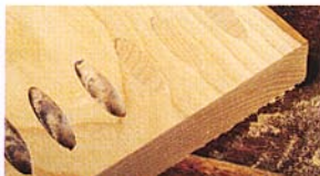
The finished plugs reveal a neat, oval cross-section
