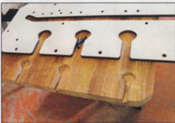
The resulting bolt holes are crisply and precisely cut, ready for installation
