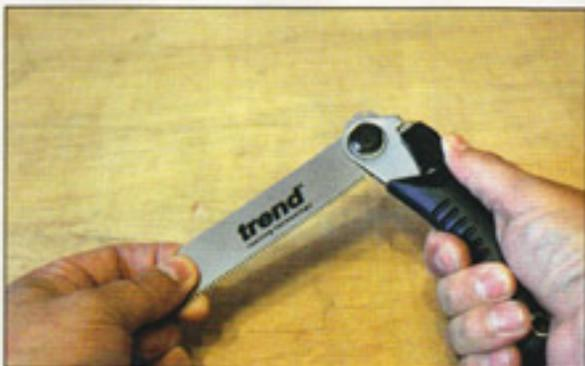
The blade folds into the handle for storage in much the same as a penknife
