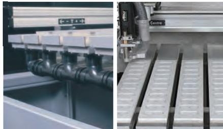
Vacuum table for CNC/PLUS/T10 and CNC/SMARTFAST machines.
