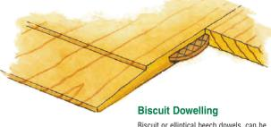
Biscuit or elliptical beech dowels, can be used to reinforce edge-to-edge panel joints. The dowels are set into semicircular recesses cut with the router fitted with a suitable grooving cutter (See Trend Biscuit Cutter Set, Ref. 342). The dowel positions are carefully set out at approx 150mm centres along the joint faces, but carefully avoiding the width of the panel raising mould at each end of the panel.
