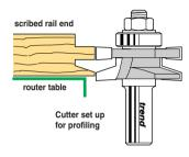
11 Ensure the fence is aligned with the bearing using a steel rule as before.
