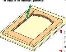
Clamp the dry assembled door frame over a piece of 6mm thick sheet material (plywood, MDF etc.) and check that it is square and flat.
