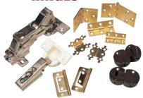
The size and type of hinge chosen will depend on the size and weight of the door itself. With flap hinges the thickness of the door style in relation to the flap width will dictate the hinge size used. Economy lay-on hinges are only suitable for lightweight doors up to 450mm wide. Concealed hinges will support larger and heavier doors and are fully adjustable once fitted.
