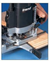
Edge moulding using a side fence.
