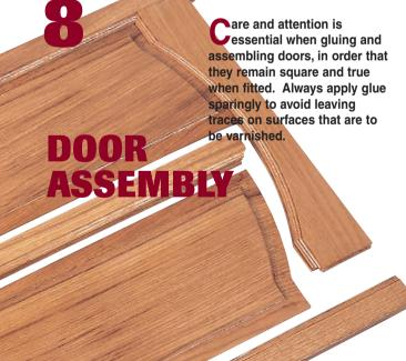
Before gluing the work together, assemble the frame dry and mark each piece of each joint for easy reference.
