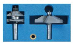
Trend panel door sets each consist of one profile scriber cutter and one matching raised panel cutter. The 1/2" shank sets are intended for use in heavy duty routers. The 8mm shank cutters can be used in routers over 750 watts, fitted with a 8mm collet. There are maximum speed constraints on the following 1/2" shank panel cutters.
