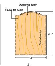
Panel margins for calculating overall panel sizes when using profile scribing cutter fitted with either 46 or 41mm groovers.
