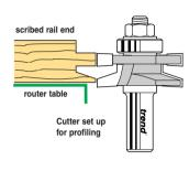
1 Ensure the fence is aligned with the bearing using a steel rule as before.
