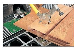
If your table is fitted with a sliding mitre fence, it is still advisable to use a workholder of this type to support the workpiece, rather than holding it against the face of the mitre fence.
