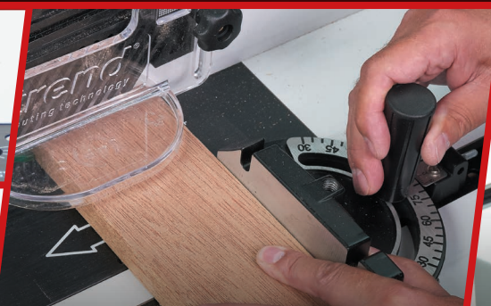
Mitre fence for jointing and moulding on end grain or angled work
