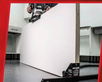
Support for routing hinges & mortises.
