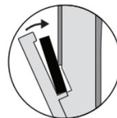
Holding the ends of the diamond stone, unclip it from the front plate magnet.
