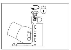
To position the fence at the 1.4mm setting, slide the rods into the deeper recesses, as shown below and tighten the fence cheeks locking knobs.
