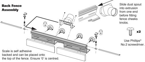
Scale can be trimmed to the length of the back fence.
