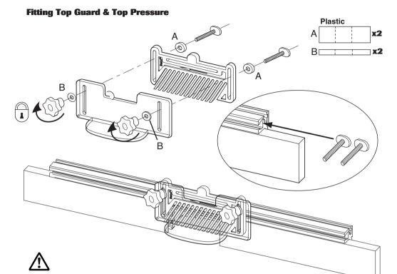
NOTICE: For some applications the thick and thin washer can be swapped over. For example, when profile scribing using a pushblock.
