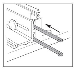
The rods can be parked in the T-slots in the top of the back fence. The rods are held by tightening the knobs.
