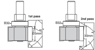
Diagrams show the technique for machining a wider groove to accept wider strip.
