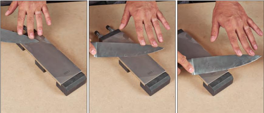
**NOTE:** For a sharper “filleting edge”, slightly decrease the cutting angle. For a “boning edge” slightly increase the angle. As a rule, High Carbon Steel knives will hone with a few passes. HSS knives and other hard steels will typically take a few extra passes. Always relax, take your time and let the diamond do the work!
