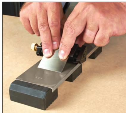
Dry the plane blade or chisel on a soft cotton cloth then apply honing compound bar\* to the rough side of leather strop. Lay the blade flat on its backside against the honing compound and with blade edge away from you pull the blade towards you
