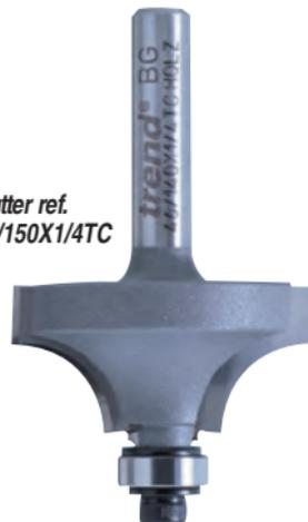
**2.** A bull-nose moulding will be required on three of the edges. For 1" (25.4mm) thick board, use a 1/2" (12.7mm) radius rounding-over cutter, Trend ref. 46/150X1/4TC or similar. Adjust the height of the cutter so that the top quirk is just clear of the top surface. The roller bearing fitted to the end of the cutter acts as the guide and runs along the centre of the board edge.
