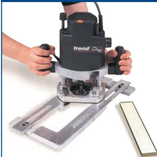
The Trend Letterbox Jig is an ideal adjustable template system for routing recesses in doors quickly and accurately. The jig has a size-adjusting device which ensures the template aperture is always square. Produced from aluminium, it will cater for apertures from 210 to 310mm long and from 46 to 82mm wide.
