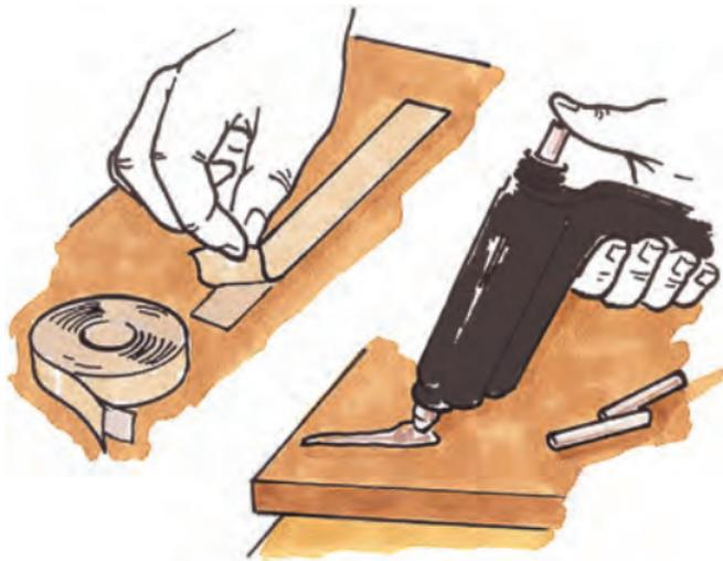
**3.** In situations where clamps or other mechanical devices are impractical, pins may be used. Where these may spoil the workpiece, double-sided tape or hot-melt glue can be used. This will only work if the material is flat, clean and dust-free.
