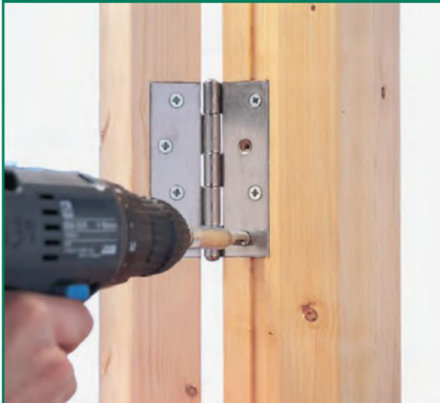
The Trend Snappy quick release drill system includes drill bit guides for quick drilling of fittings for hinges, drawer runners and other ironmongery pre-drilled with countersunk holes.
