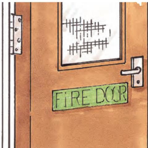
Often doors and frames in domestic and industrial applications are subject to fire regulations and are graded according to their construction with a fire rating. Safety regulations specify the fitting of intumescent strips and smoke-seals. These have to be recessed in order not to interfere with the operation of the door.
