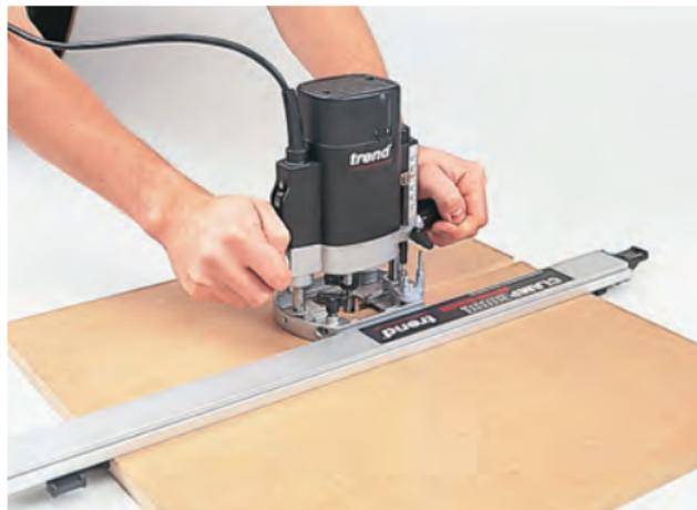
3. Loosely fit a Clamp Guide, adjust door jambs ensuring marked grooves run parallel to each other.
