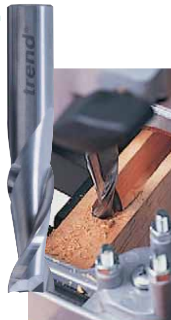
Up-cut spirals remove the waste, but leave a slightly ragged edge.
