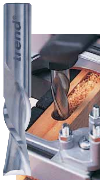
Down-cut spirals give a clean sharp edge but compact the waste in the mortise.
