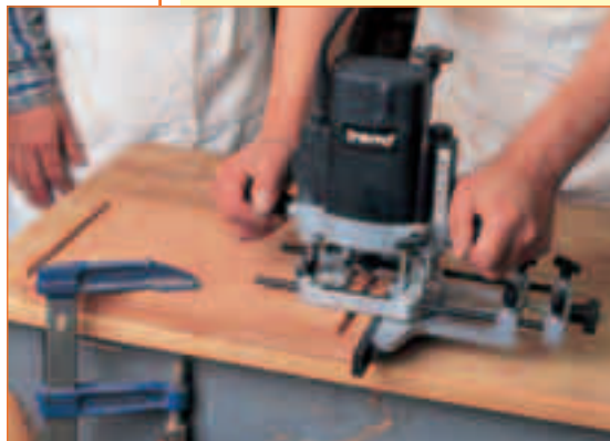
Producing housings for drawer frame
