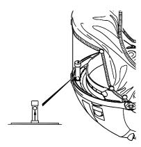
Press the red on/off switch to operate the fan. The red ball is raised to the top of the indicator tube if the system is operating correctly.
