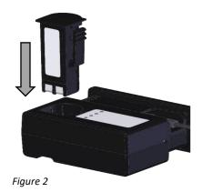
Insert the battery as shown in Figure 2. Ensure the battery fully 'clicks' into position.
