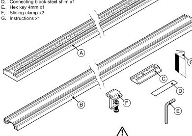
The scale is self adhesive backed. Only remove a 20mm section of the self adhesive backing to ease positioning, alternatively the scale can be slid on to the other extrusion to any position.
