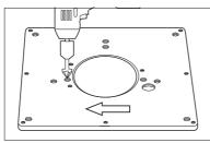
Countersink the hole with a countersink bit to a depth so the heads of the screws are slightly below the top surface. Clean off any burrs created
