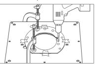
■ Ensuring that the drill bit will not foul any webbing or fixtures on the router base, drill with a 6mm diameter metal cutting drill bit into the insert plate and through the router base two holes.
