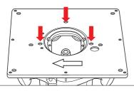
■ Remove insert plate and mark the centre of the holes with a centre punch.
