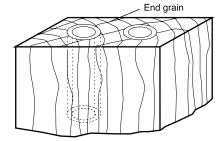
The plug can be removed from the timber by cutting across timber with a handsaw or bandsaw at the correct height.
