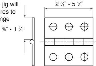
Example of hinge positions possible using a 4 1/2" hinge and a 7' 11" door and 8' frame.
