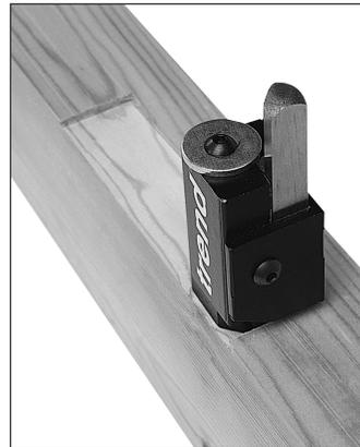
After use, loosen jointing plate fixing screws to disassemble and store jig carefully.
