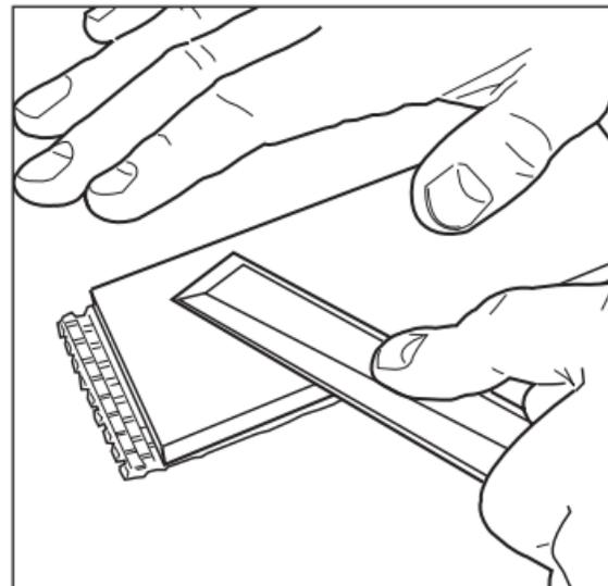
2. Lay leather strop out flat with the rough side uppermost.
