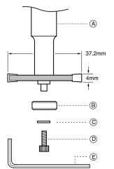
The set is supplied assembled with the B127A ball bearing fitted. Dependant on the biscuit size used, the relevant ball bearing should be fitted onto the cutter, this bearing will then automatically set the depth of groove.
