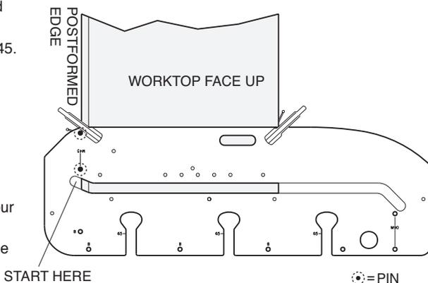
**Cutting Bolt Recess Slots for
