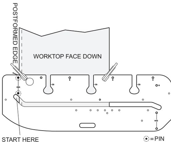
**Cutting Bolt Recess Slots for Male 90° Connecting Bolt**
