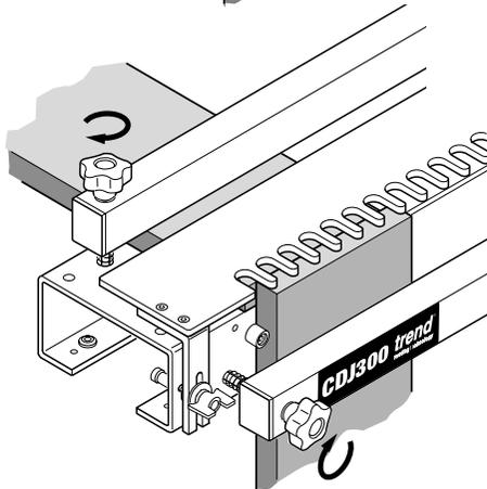
**Clamping Bars and Knobs**
