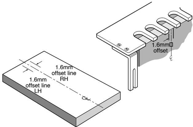
**Box comb joint too shallow = increase depth adjustment of cutter**
