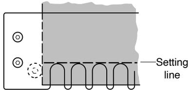
A packing piece the same thickness as the timber being clamped in the top clamp should be used to support the template comb.
