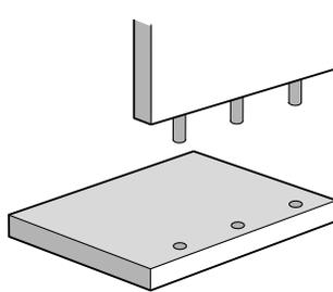
**Routing the Dowel Joint on Face of Workpiece**
