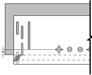
**Routing of Dowel Holes off Jig**
