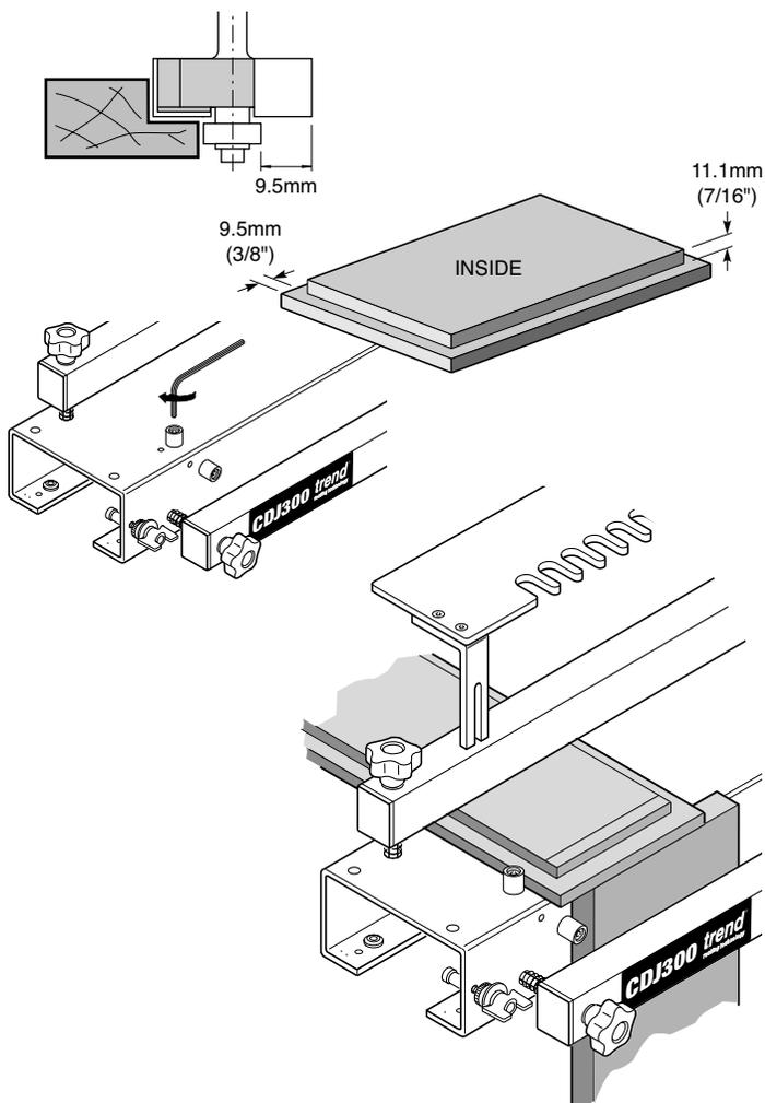
**Routing Pin Socket in the Drawer Front**
