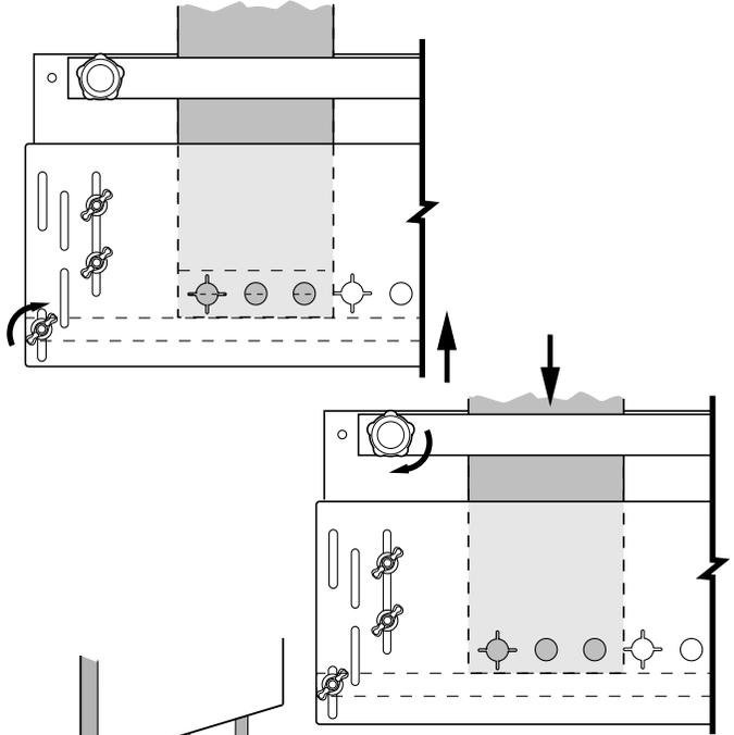
**Routing the Dowel Joint on End of Workpiece**
