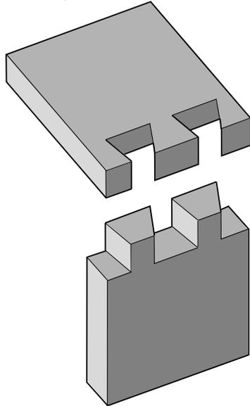
**Joint too loose = move template for pin away from jig body.**
