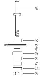
Before using cutter, please ensure it is correctly assembled and locking nut is fully tightened to correct torque setting.
