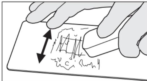
4. Rub the bevel edge sided of the blade into the paste a few times.
