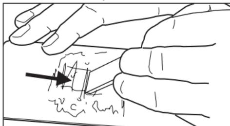
5. Polish off the surface of the tool on the clean half of the leather strop.
