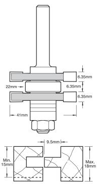
Tonque & groove joint showing minimum and maximum possible timber thickness.
